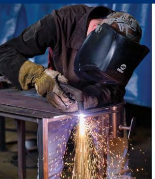
For more information on this class, contact Wendy Friesen at 402-323-5591 or wfriesen@southeast.edu This is an introduction to Gas Metal Arc Welding theory, safety, applications, manipulative skills, welding principles, and procedures. Filler wires, shielding gases, welding power sources, welding of carbon steel, and welding processes on different joint configurations are included.
